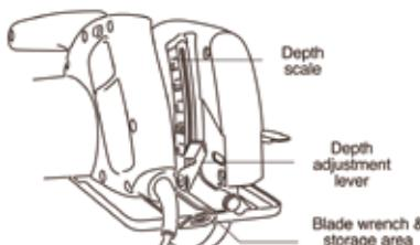
The blade should not be more than one tooth length below the material to be cut for minimum splintering.
