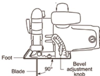
If adjustment is necessary, tilt the foot to  $45^\circ$ , tighten the bevel adjustment knob, and bend the "TAB" with an adjustable wrench or pliers.
