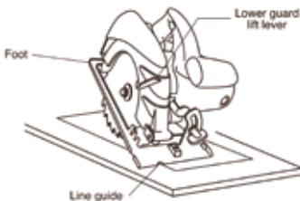
Start the motor with the blade clearing the material to be cut. Gradually lower the saw's back end using the foot's front end as the hinge point.
