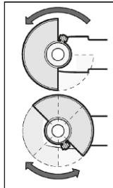
Place the protection guard on the spindle collar. Adjust the position of the protection guard to the requirements of the operation. Lock the protection guard by tightening the locking screw using a Phillips screwdriver.
