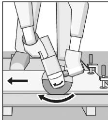
The machine must always work in an up-grinding motion. Otherwise, the danger exists of it being pushed uncontrolled out of the cut.
